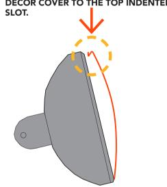
3. INSPECT OVERALL DÉCOR COVER TO MAKE SURE IT IS SNUG FIT ONTO THE THE HEATER BODY.
