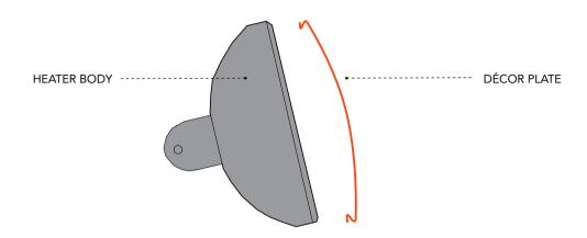
START BY INSERTING THE DÉCOR PLATE TO THE BOTTOM OF THE HEATER'S INDENTED SLOT.
