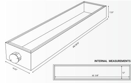
The included junction box should only be used if it remains accessible. If it is hidden or inaccessible, please bypass it and connect to the nearest accessible junction box. Our team will provide the part number for the required whip, which is available in lengths ranging from 10 ft to 75 ft.
